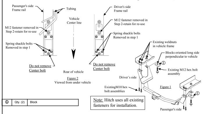
1. Remove (2) rearmost spring shackle mounting bolts, each side, as shown in Figure 2. Retain bolts for hitch installation.
